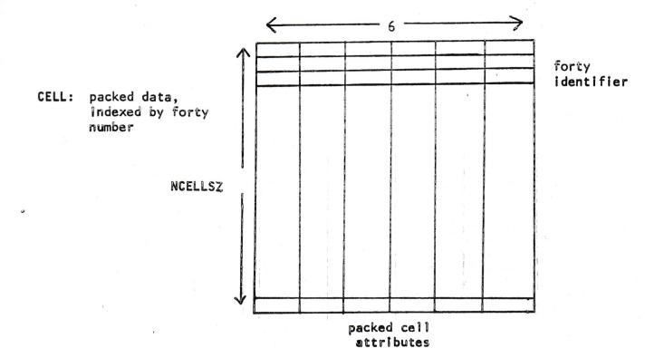
Figure 2. Cell File Structure
